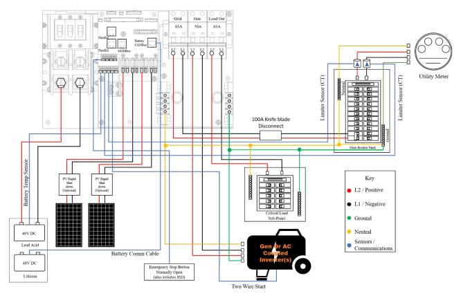
Sol-Ark 12K Load Side AC Coupled Wire Diagram 120V/240V
