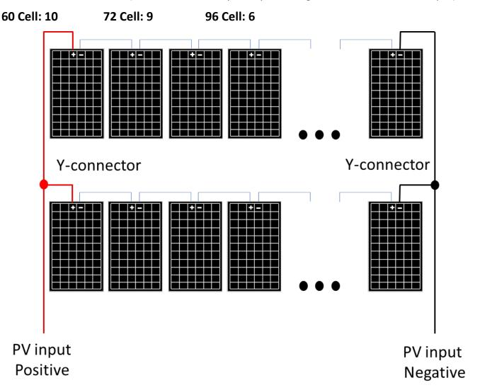
**If using Y-Connectors:** (Running two strings in parallel, totaling 20A (self-limiting) Note: separate wires can be used per string, and string minimum is usually 5 panels or 175V)
