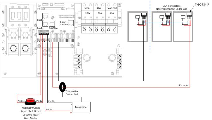
Note: The Built in 12V power supply in the user area of the Sol-Ark (Pins 15 and 16) is rated for 100mA (1.2W)
